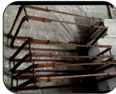
Figure 6: Steel Cage without Shear reinforcement.
