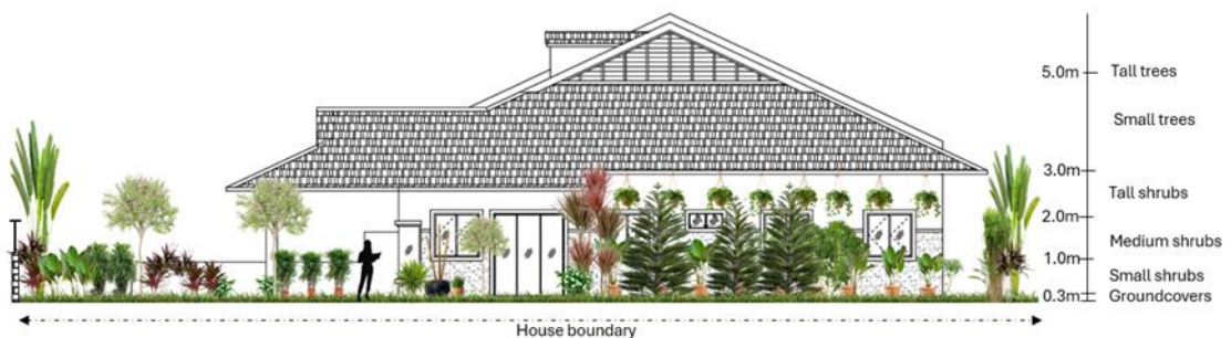
Figure 5. Side Elevation of the SLH, Featuring Layered Vegetation With Varied Heights That Enhances Lateral Shading and Improves the Microclimate Along the Building Perimeter.
