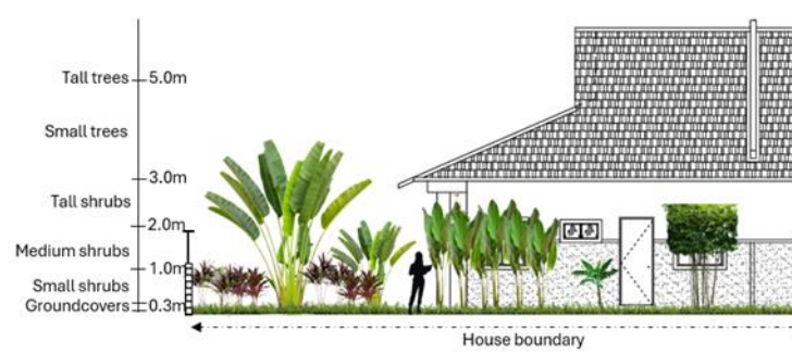
Figure 6. Rear Elevation of the SLH, Where Compact Vegetation Including Medium Shrubs and Groundcovers, Offers Minimal Shading to the Building but Contributes to Ground-Level Cooling
