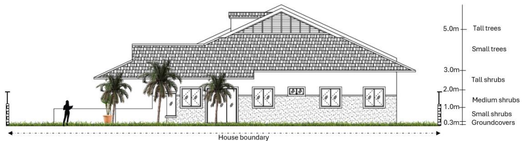
Figure 9. Side Elevation of SSLH with three Wodyetia bifurcata (2–5m), offering limited lateral shading due to sparse canopy and farther from wall
