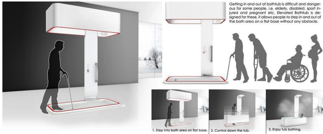
Fig. 2 Elevated Bathtub Design [33]
